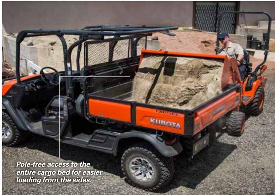
*Pole-free access to the entire cargo bed for easier loading from the sides.*
