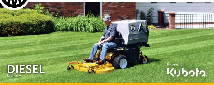
The D21d is a premium commercial GHS mower with impressive industrial power, agility and premium-quality mowing. Featuring the Kubota D722 liquid cooled, diesel engine, and a standard Grammer suspension seat, the D21d is designed for all day comfort and long machine life.
